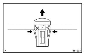
46. REMOVE COOLER (SOLAR SENSOR) THERMISTOR (AUTO AIR CONDITIONING)
