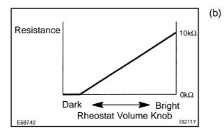
) Check the resistance between terminal 3 (RV) and terminal 4 (T) when operating the light control rheostat volume knob. Also, check that the resistance changes continuously.
