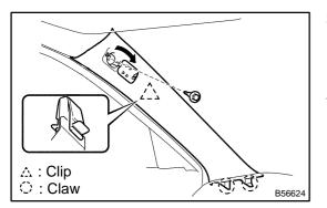
33. REMOVE FRONT PILLAR GARNISH LH (W/ CURTAIN SHIELD AIR BAG)
