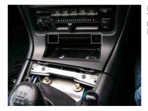
Firstly remove the ashtray, gear lever gaiter and its plastic surround. The plastic surround is a snap fit, just pull it up gently at the back. Lowering the steering gives you more room later on. Remove the 2 screws from behind the ashtray
