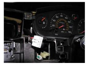
Remove the narrow trim above the cluster. You will now be able to remove the instrument cluster (reaching behind to unplug the various connectors). You'll find it easier to withdraw the cluster with the steering column set to its lowest position.
