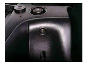
Pull the stereo surround off (snap fit) and reach behind to unplug the cigarette lighter power plug and hazard light switch plug. The cigarette lighter illumination bulb holder twists 90 degrees to allow removal. As you can see from the picture below, the hazard switch connector (larger white connector) has a security clip. This clip hides on the tight side (nearest the instruments and away from your eyes).
