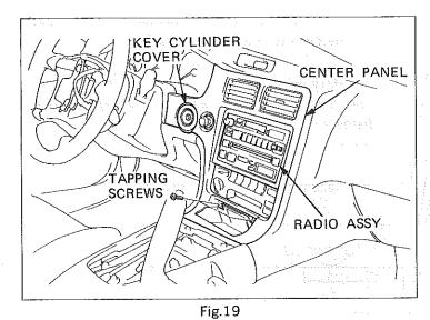
(b) Temporarily remove the key cylinder cover, center panel and radio assy.
