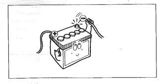
(1) Disconnect the ground cable at the battery negative terminal.
