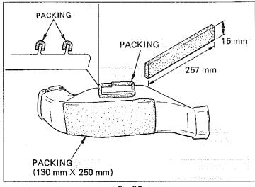
(e) Attach the two pieces of packing to the air duct.
