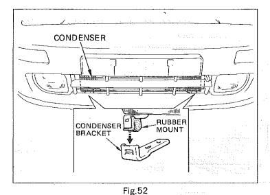
(k) Locate the condenser brackets into the rubber mounts of the condenser.
