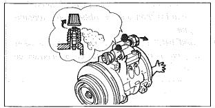
(3) Installing air conditioning lines and A/C harnesses. route properly to avoid interference with surrounding parts.
