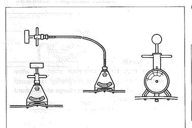
(3) Installing the drive belt, check the belt tension using NIPPONDENSO BTG-20 or BURROUGHS BT-33-73F.
