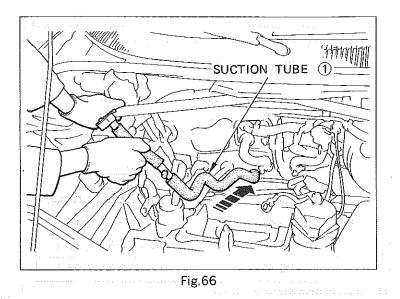
(e) Pass the suction tube ① through the bulkhead as shown.
