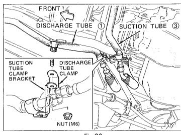
(k) Fasten the discharge tube ① and the suction tube 3 to the frame using a nut.
