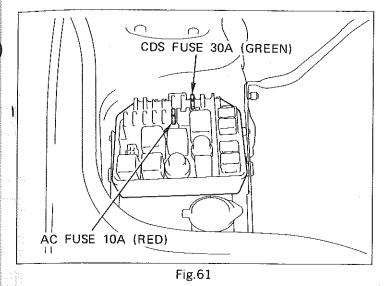
(b) Install the two fuses to the relay box.
