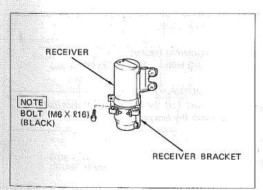
(b) Assemble the receiver to the receiver bracket.
