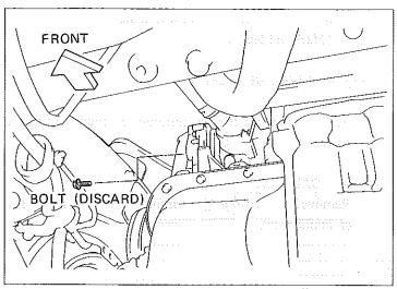
(c) Remove and discard the original bolt from the engine block.
