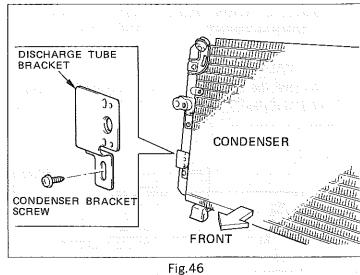
(c) Install the discharge tube bracket to the condenser using the condenser bracket screw.
