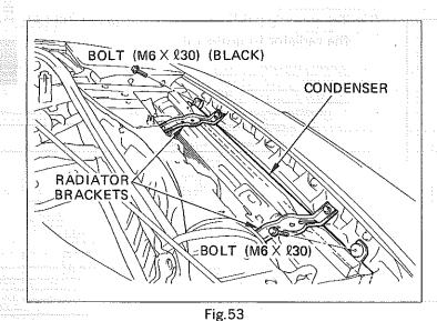
(I) Fasten the condenser to the frame using two bolts.
