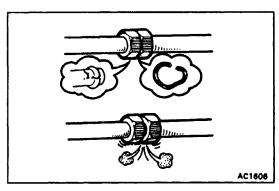
• Tighten the O-ring fittings or the bolted type fittings to the specified torque.
