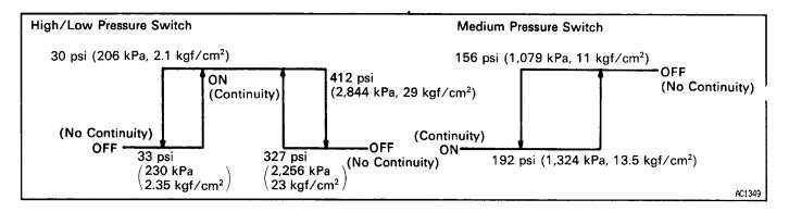
If defective, replace the pressure switch.
