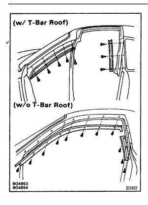
2. REMOVE ROOF DRIP SIDE FINISH FRONT MOU-LDING
