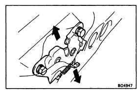
3. ADJUST LUGGAGE COMPARTMENT DOOR LOCK Adjust the lock by loosening the bolts.
