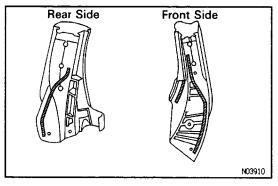
(b) Install the seal to the weatherstrip.
