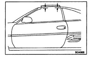
(b) Check for a difference in level between the removable roof glass and the roof panel.
