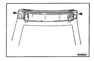
**6. REMOVE SIDE RAIL WEATHERSTRIP** Remove two screws and the weatherstrip.
