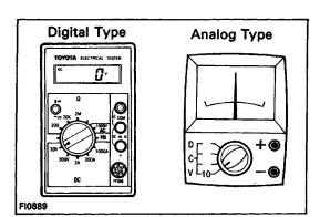
(c) Use a volt/ohmmeter with high impedance (10k/V minimum) for troubleshooting of the electrical circuit.
