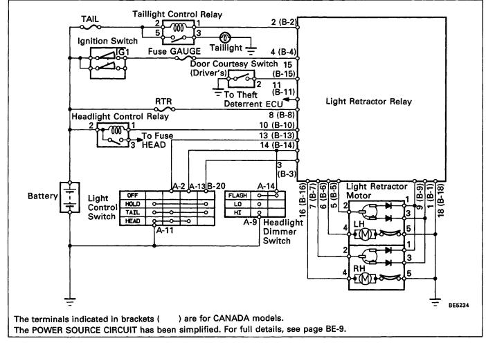
• Current flows from the battery to terminal 8 (B-8) of the light retractor relay.
