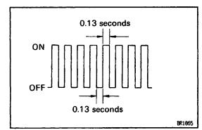
(d) Check that the ABS warning light blinks. HINT: If the ABS warning light does not blink, inspect the ABS warning light circuit.
