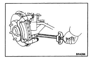
(e). (n this position, if the runout is within specification, install the torque plate and torque the mounting bolts.
