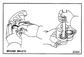
3. INSTALL PISTON SEALS AND PISTONS IN CYLIN-DER
