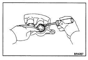
4. INSTALL CYLINDER BOOTS AND CYLINDER BOOT SET RINGS
