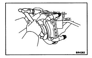
(b) Using a chisel and hammer, tap out the two dust boots.
