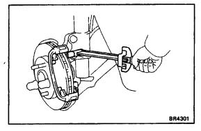
(e) In this position, if the runout is within specification, install the torque plate and torque the mounting bolts.
