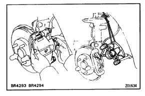
(b) Remove the brake cylinder and suspend it so the hose is not stretched.
