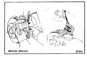
(c) Remove the brake cylinder and suspend it so the hose is not stretched.
