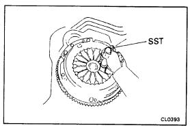
If alignment is not as specified, using SST, adjust the diaphragm spring tip alignment. SST 09333-00013
