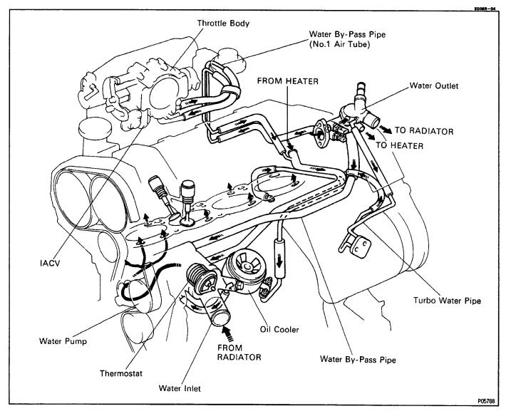
The cooling system is composed of the water jacket (inside the cylinder block and cylinder head), radiator, water pump, thermostat, electric fan, hoses and other components.
