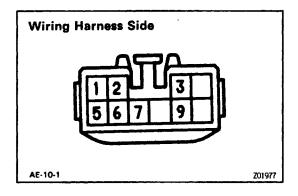
(b) Check the connector on the wiring harness side as shown in the chart.
