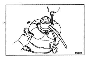
(b) Remove the three screws, rubber bushings, steel plate bushings and motor.
