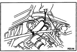
3. REMOVE NO.2 INTAKE AIR CONNECTOR
