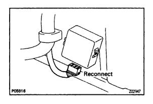
(c) Reconnect the fan control module connector.
