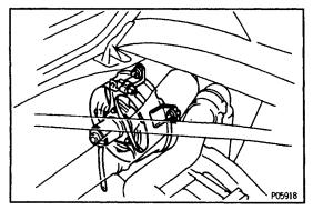
(e) Reinstall the engine compartment temperature sensor with the two bolts.
