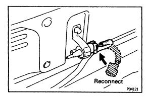
(f) Reconnect the engine compartment temperature sensor.
