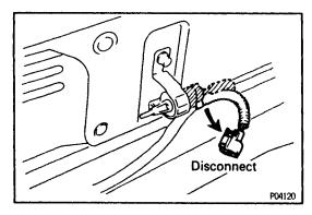
(c) Disconnect the engine compartment temperature sensor.
