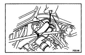
2. INSTALL NO.2 INTAKE AIR CONNECTOR
