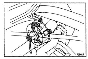
(b) Check that the cooling fan stops.
