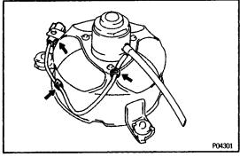
(b) Install the wire and connector to the fan shroud.
