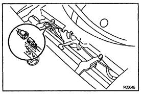
(b) Connect the cooling fan connector.
