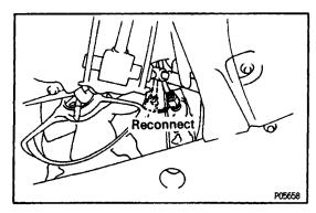
(e) Reconnect the engine coolant temperature sensor.
