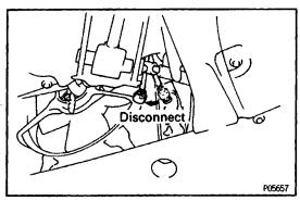
(c) Disconnect the engine coolant temperature switch.
