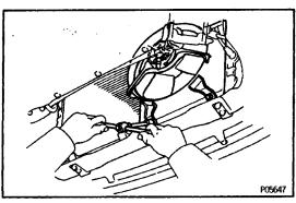
(b) Remove the three bolts and cooling fan.
