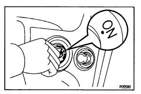
On–Vehicle Inspection 1. INSPECT COOLING FAN OPERATION AT LOW TEMPERATURE (Below 85°C (185°F)) (a) Turn the ignition switch ON.
