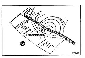
2. REMOVE UPPER RADIATOR SUPPORT SEAL(a) Disconnect the hood weatherstrip.
