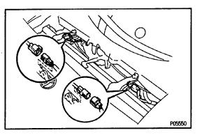
(b) Connect the two cooling fan connectors.
