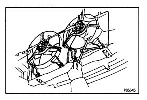
(b) Remove the three bolts and cooling fan. Remove the two cooling fans.
