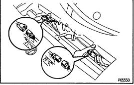
(a) Disconnect the two cooling fan connectors.
