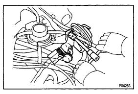
(c) Loosen the union nut, and Remove the two bolts, EGR valve and gasket.
