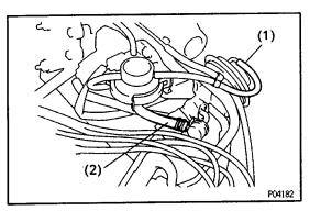
(b) Connect the following hoses to the EGR valve:(1) Vacuum hose (from vacuum modulator)(2) EGR hose (from vacuum modulator)
