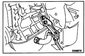
(d) Install the RH TWC stay with the four bolts.
