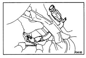
10. REMOVE FRONT EXHAUST PIPE (See step 2 in Main TWC Replacement)
