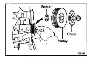
(e) Temporarily install the spacer, pulley and pulley cover with the nut.
