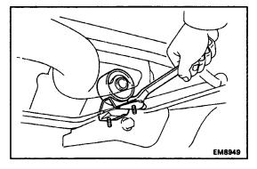
(c) Install the support bracket with the two bolts.
