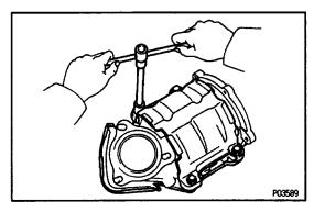
(d) Remove the nine bolts and two heat insulators from the TWC.
