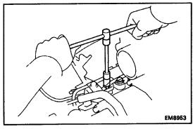
(b) Remove the two bolts holding the clutch release cylinder to the transaxle.
