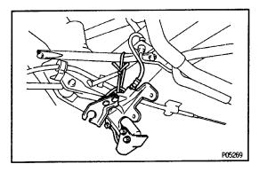
HINT: Suspend the clutch release cylinder to the suspension brace with a string.
