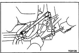
(i) Install the suspension brace with the two bolts.
