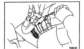
(d) Tighten the two bolts of the lower side of the A/C compressor.
