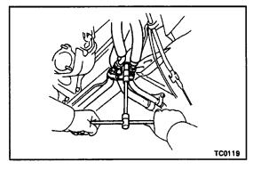
(h) Install the two A/C pipes with the nut.
