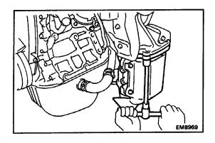
(c) Install the TWC with the three bolts and two nuts.
