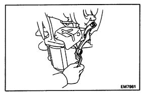
(e) Install the LH TWC stay with the three bolts.
