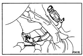
17. REINSTALL FRONT EXHAUST PIPE (See step 3 in Main TWC Replacement)
