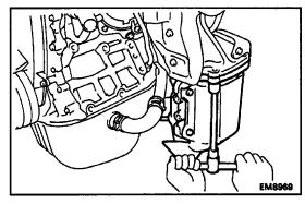
(c) Remove the three bolts, two nuts, TWC, gasket, retainer and cushion.
