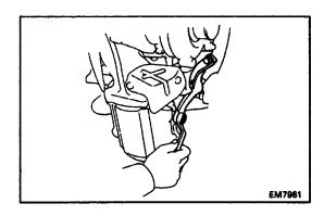
(b) Remove the three bolts and LH TWC stay.
