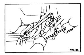
(b) Remove the two bolts and suspension brace.
