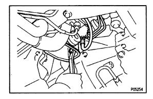
(c) Tighten the two bolts holding the clutch release cylinder to the transaxle.
