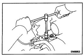
(b) Install the clutch release cylinder with the two bolts.
