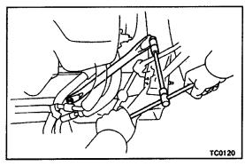
(i) Install the lower suspension brace with the two bolts. Torque: 73 N-m (740 kgf-cm, 64 ft-lbf)
