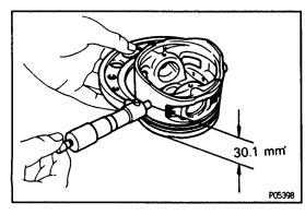
(a) Using a micrometer, measure the piston diameter at ring angles to the piston pin center line, 30.1 mm (1.185 in.) from the piston head.
