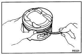
(b) Using a groove cleaning tool or broken ring, clean the piston ring grooves.
