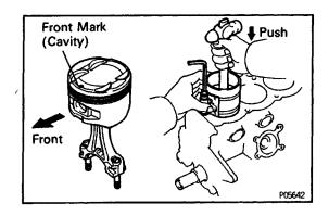
(b) Using a piston ring compressor, push the correctly numbered piston and connecting rod assemblies into each cylinder with the front mark of the piston facing forward.
