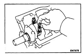
(d) Cover the connecting rod bolts with a short piece of hose to protect the crankshaft from damage.
