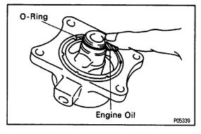
(b) Apply a light coat of engine oil on the small O-ring.
