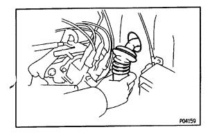
(b) Pull out the engine wire from the luggage compartment.
