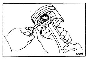
(e) Using a small screwdriver, Install a new snap ring on the other side of the piston pin hole.
