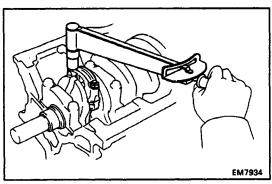
(h) Install the connecting rod cap.
