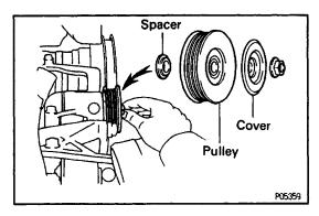
(e) Temporarily install the spacer, idler pulley and pulley cover with the nut.
