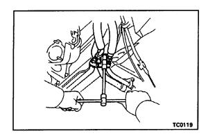
(h) Install the A/C pipes with the two clamps and nut.
