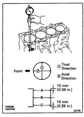
Using a cylinder gauge, measure the cylinder bore diameter at positions A, B and C in the thrust and axial directions.
