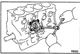
(c) Install the oil cooler bracket with the four bolts.
