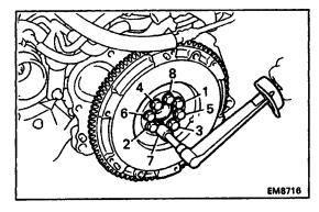
(b) Install the flywheel on the crankshaft.
