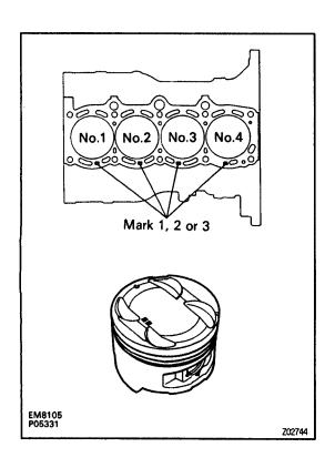
If the oil clearance is greater than maximum, replace all the four pistons and rebore all the four cylinders. If necessary, replace the cylinder block.
