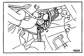
(b) Remove the two bolts and mounting bracket. Disconnect the clutch release cylinder from the transaxle.
