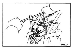
(b) Remove the through bolt, nut, three bolts and LH mounting insulator.
