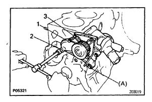
(b) Install the water pump with the three bolts. Tighten the bolts in the sequence shown.
