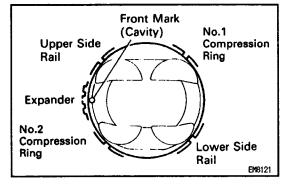
(c) Position the piston rings so that the ring ends are as shown.
