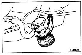
HINT: Suspend the A/C compressor to strut rod with a string.
