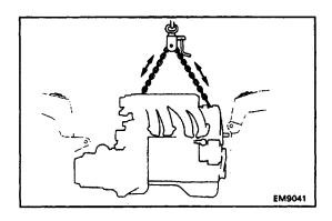
(c) Keep the engine level, and align RH and LH mounting with the body mountings.
