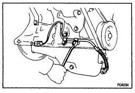
(b) Remove the two bolts and sensor wire.
