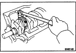
(c) Using a plastic–faced hammer, lightly tap the con– necting rod bolts and lift off the connecting rod cap. HINT: Keep the lower bearing inserted with the connecting cap.
