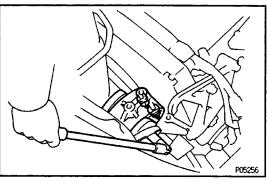
(c) Remove the through bolt, two nuts and RH mounting insulator.
