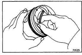
(b) Remove the two side rails and oil ring by hand.
