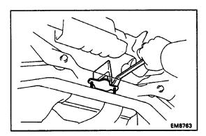
(d) Install the damper with the two bolts.
