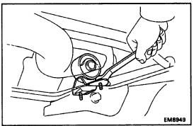
(c) Install the support bracket with the two bolts.
