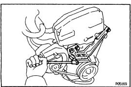
5. REMOVE RH ENGINE MOUNTING BRACKET
