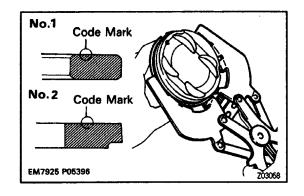
(b) Using a piston ring expander, install the two compression rings with the code mark facing upward.
