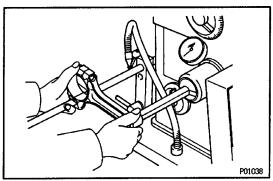
(d) Using a pin hole grinder, hone the bushing to obtain the standard specified clearance (see step B above) between the bushing and piston pin.
