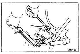
(h) Tighten the through bolt holding the LH mounting insulator to the body.
