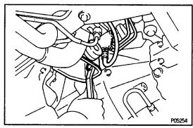
(c) Tighten the two bolts holding the mounting bracket to to the transaxle.
