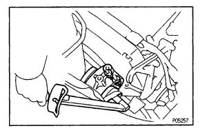
(i) Tighten the two nuts holding the RH mounting insulator to the mounting bracket.
