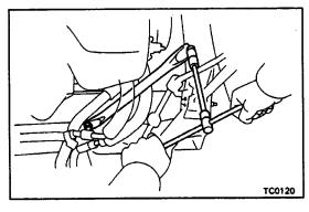
(b) Remove the two bolts and lower suspension brace.
