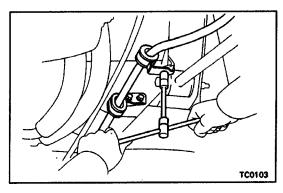
(j) Install the parking brake cable with the two clamp and three bolts.
