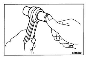
(e) Check the piston pin fit at normal room temperature. Coat the piston pin with engine oil, and push it into the connecting rod with your thumb.
