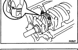
(b) Remove the connecting rod cap nuts.
