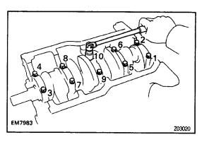
(b) Using two screwdrivers, pry out the main bearing cap, and remove the main bearing caps, lower bearing and remove the main bearing caps, lower bearings and lower and lower thrust washers (No.3 main bearing cap only).
