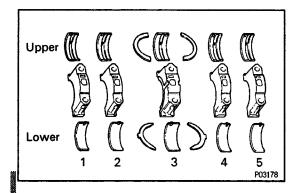
HINT: Arrange the main bearing caps, bearings and thrust washers in correct order.
