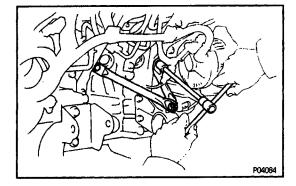
(b) Install the bearing bracket stay with the two bolts and nut.
