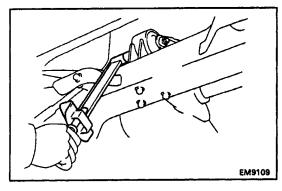
(d) Tighten the through bolt holding the mounting insulator to the mounting bracket.
