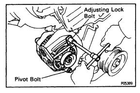
(c) Remove the pivot bolt and adjusting lock bolt, and disconnect the alternator from the bracket.
