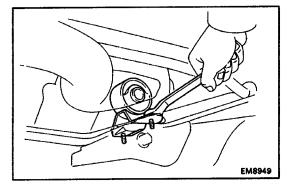
(b) Remove the two bolts and support bracket.
