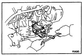
(b) Remove the two bolts and bearing bracket.
