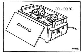
(b) Gradually heat the piston to  $80 - 90^{\circ}\text{C}$  (176 - 194° F).
