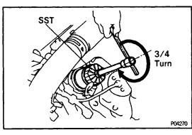
(e) Using SST, give it an additional 3/4 turn to seat the filter.
