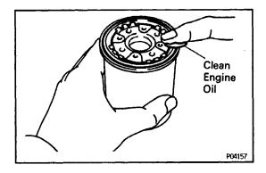
(c) Lubricate the filter rubber gasket with clean engine oil.
