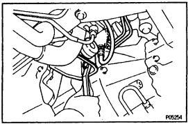
(c) Tighten the two bolts holding the clutch release cylinder to the transaxle.
