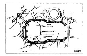
(d) Remove the seventeen bolts and two nuts.
