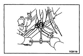
(h) Install the two A/C pipes with the two clamps and nut.
