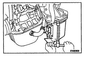
(b) Install the TWC with the three bolts and two nuts.
