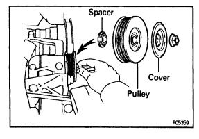
(e) Temporarily install the spacer, pulley and pulley cover with the nut.
