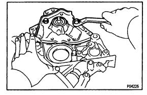
(c) Install the oil pump body cover with the two bolts.
