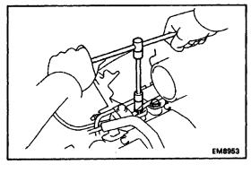
(b) Install the clutch release cylinder with the two bolts.
