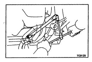
(i) Install the lower suspension brace with the two bolts.
