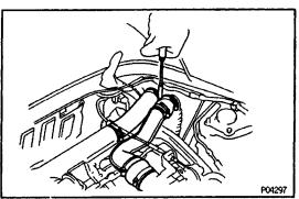
18. INSTALL NO.1 AND NO.2 INTAKE AIR CONNECTORS
