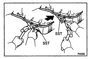
(e) Insert the blade of SST between the cylinder block and oil pan, and cut off applied sealer and remove the oil pan.
