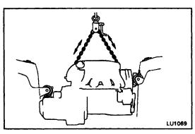
19. SUSPEND ENGINE WITH ENGINE SLING DEVICE
