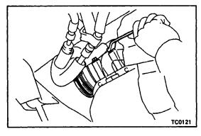
(i) Remove the two bolts, and disconnect the A/C compressor from the engine.
