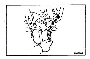
(d) Install the LH TWC stay with the three bolts.
