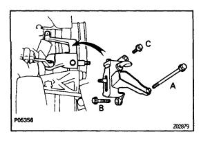
(b) Install the idler pulley bracket with the three bolts.
