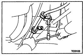
(j) Install the parking brake cable with the two clamps and three bolts.
