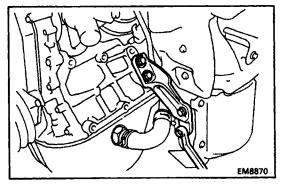
(c) Install the RH TWC stay with the four bolts.
