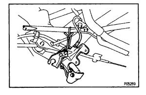
HINT: Suspend the clutch release cylinder to the suspension brace with a string.
