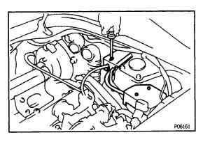
8. (w/ CRUISE CONTROL SYSTEM) REMOVE CRUISE CONTROL ACTUATOR AND ACCELERATOR LINKAGE
