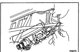
(b) Remove the two bolts and No.4 air tube.
