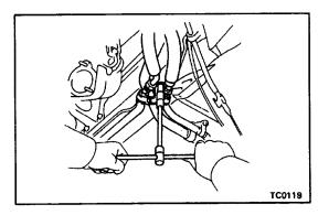
(c) Remove the clamp nut, and disconnect the two A/C pipes.
