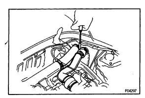
7. INSTALL NO.1 AND NO.2 INTAKE AIR CONNECTORS
