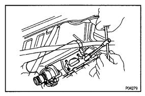
(b) Install the No.4 air tube with the two bolts.
