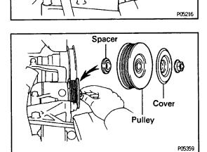
(f) Remove the nut, pulley cover, idler pulley and spacer.
