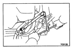
(b) Remove the two bolts and suspension brace.
