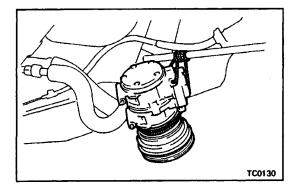
HINT: Suspend the A/C compressor to strut rod with a string.
