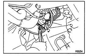
(c) Tighten the two bolts holding the clutch release cylinder to the transaxle. Torque: 77 N-m (790 kgf-cm, 57 ft-lbf)
