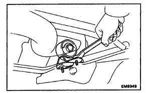
(b) Remove the two bolts and support bracket.
