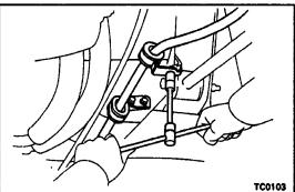
(j) Install the parking brake cable with the two clamps and three bolts.
