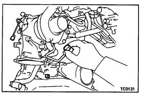
(b) Install the oil pipe with the bolt, two new gaskets and union bolt. Do not torque the bolt and union bolt.
