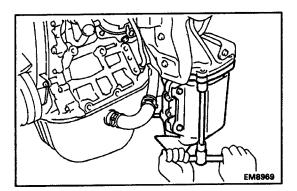
(b) Install the TWC with the three bolts and two nuts. Torque: 29 N-m (300 kgf-cm, 22 ft-lbf)
