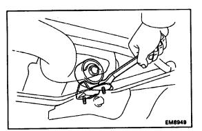
(c) Install the support bracket with the two bolts. Torque: 21 N-m (210 kgf-cm, 15 ft-lbf)
