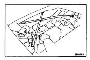
5. REMOVE UPPER SUSPENSION BRACE Remove the two bolts, two nuts and upper brace.
