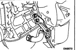
**15. REMOVE MAIN TWC** (a) Remove the four bolts and RH TWC stay.
