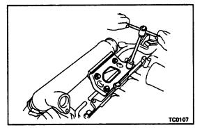
(b) Install the air tube stay with the four bolts. Torque: 19 N-m (195 kgf-cm, 14 ft-lbf)
