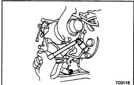
(e) Tighten the union bolt holding the oil pipe to the cylinder block.
