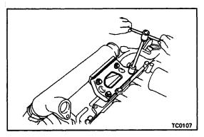
**19. REMOVE NO.4 AIR TUBE**(a) Remove the four bolts and air tube stay.
