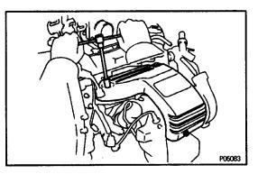
**10. INSTALL TURBOCHARGER HEAT INSULATOR** Install the heat insulator with the three bolts.
