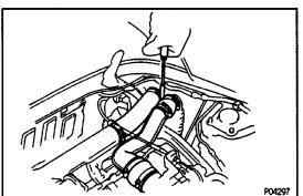
25. INSTALL NO.1 AND NO.2 INTAKE AIR CONNECTORS
