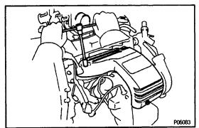
21. REMOVE TURBOCHARGER 'HEAT INSULATOR Remove the three bolts and heat insulator.
