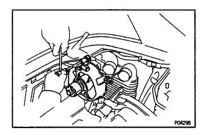
23. INSTALL ENGINE COMPARTMENT COOLING FAN(a) Install the cooling fan with the three bolts.(b) Connect the cooling fan connector.
