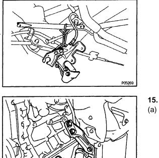
HINT: Suspend the clutch release cylinder to the suspension brace with a string.
