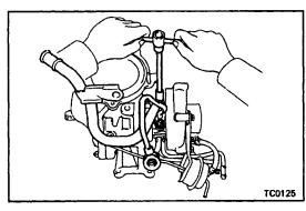
27. REMOVE TURBO OIL PIPE Remove the two nuts, oil pipe and gasket.
