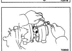
**29. REMOVE SIDE BEARING HOUSING PLATE** Remove the two nuts, housing plate and gasket.
