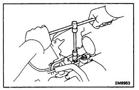
(b) Remove the two bolts holding the clutch release cylinder to the transaxle.
