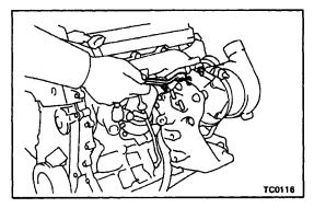
(b) Remove the four nuts, turbocharger and gasket.
