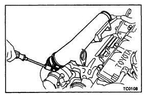
(b) Loosen the hose clamp, and remove the air tube.
