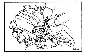
**20. REMOVE RH FRONT ENGINE HANGER** Remove the four bolts and engine hanger.
