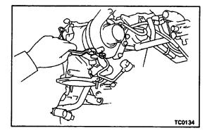
(d) Tighten the two nuts holding the oil pipe to the turbocharger. Torque: 17 N-m (175 kgf-cm, 13 ft-lbf)
