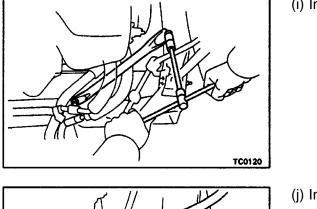
(i) Install the lower suspension brace with the two bolts. Torque: 73 N-m (740 kgf-cm, 54 ft-lbf)
