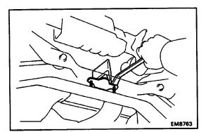
(d) Install the damper with the two bolts. Torque: 21 N-m (210 kgf-cm, 15 ft-lbf)
