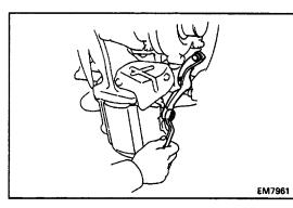
(d) Install the LH TWC stay with the three bolts. Torque: 59 N-m (600 kgf-cm, 43 ft-lbf)
