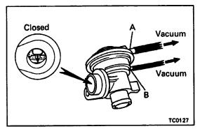
(b) In the preceding condition, apply vacuum to port B, and check that the valve is closed.
