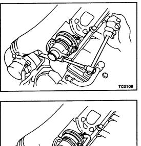
(c) Install the air by-pass valve with the bolt. Torque: 19 N-m (195 kgf-cm, 14 ft-lbf)
