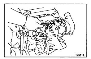
(c) Tighten the four nuts holding the turbocharger to the exhaust manifold. Torque: 64 N-m (650 kgf-cm, 47 ft-lbf)
