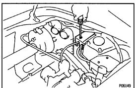
7. (w/ CRUISE CONTROL SYSTEM) REMOVE CRUISE CONTROL ACCELERATOR LINKAGE
