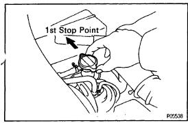
(g) Fasten the radiator (water filler) cap to the 1st stop point.
