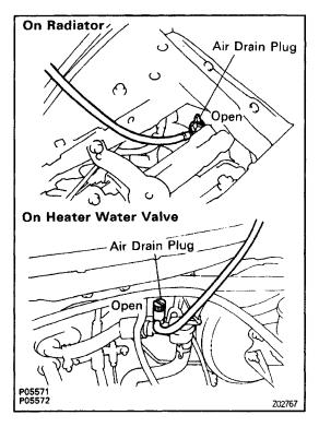
(b) Open the air drain plugs of the radiator or heater water valve above three turns.
