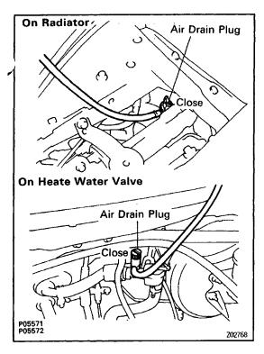
(f) When the coolant level in the air drain service hoses stops dropping, close the air drain plugs of the radiator and heater water valve.
