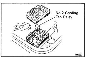
No.2 Cooling Fan Relay ("FAN NO.2") **NO.2 COOLING FAN RELAY INSPECTION** 1. REMOVE NO.2 COOLING FAN RELAY
