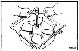
2. INSTALL FAN Install the fan with the nut.
