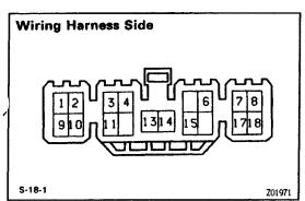
(c) Check the connector on the wiring harness side as shown in the chart.
