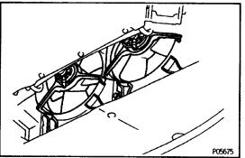
(b) Check that the cooling fans stops.If not, check the cooling fan relays and ECTS, and check for a concrete or severed wire by
