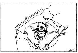
**COOLING FAN ASSEMBLY** (See Components for Disassembly and Assembly) 1. INSTALL FAN MOTOR
