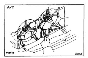
(c) (A/T) Remove the three bolts and cooling fan. Remove the two cooling fans.
