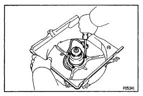
(b) Remove the three screws and fan motor.
