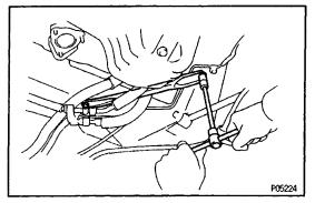
(b) Remove the two bolts and lower suspension brace.
