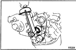
(a) Install the pulley with the bolt.
