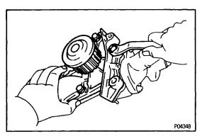
11. REMOVE WATER PUMP FROM WATER PUMP COVER
