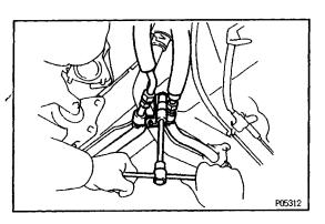
(g) Install the A/C pipes with the two clamps and nut.
