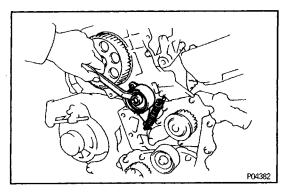
**8. REMOVE TIMING BELT TENSION SPRING** Loosen the No.1 idler pulley bolt, and remove the tension spring.
