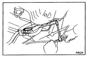
(h) install the lower suspension brace with the two bolts. Torque: 73 N-m (740 kgf-cm, 54 ft-lbf)
