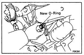
2. INSTALL WATER PUMP AND WATER PUMP COVER ASSEMBLY
