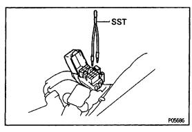
9. REMOVE SST FROM DATA LINK CONNECTOR 1 SST 09843-18020 IF NO PROBLEM IS FOUND WITH THIS INSPECTION, SYSTEM IS NORMAL; OTHERWISE INSPECT EACH PART
