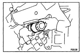
(d) Tighten the oil filter by hand until the rubber gasket contacts the seat of the filter mounting.
