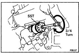
(e) Using SST, give it an additional 3/4 turn to seat the filer.
