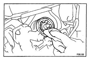
(b) Clean the oil filter contact surface on the oil filter mounting.
