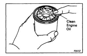
(c) Lubricate the filter rubber gasket with clean engine
