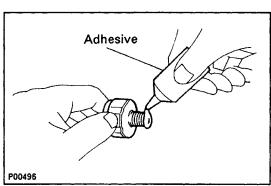
3. REMOVE OIL PRESSURE SWITCH, AND INSTALL OIL PRESSURE GAUGE
