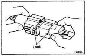
(b) Fully insert the connector and check that it is locked.
