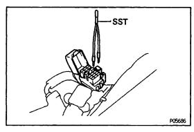
(e) Remove the SST from the data link connector 1. SST 09843–18020
