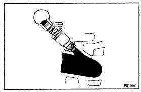
4. Install the injector– to delivery pipe and cylinder head as shown in the illustration.
