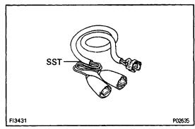
Use SST for inspection or test of the injector or its wiring connector. SST 09842–30070
