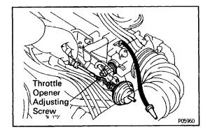
(e) Adjust the throttle opener setting speed by turning the throttle opener adjusting screw.
