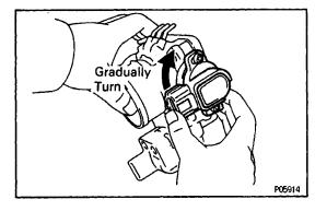
(e) Gradually turn the sensor clockwise until the ohmmeter deflects, and secure it with the two set screws.
