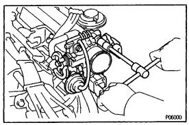
(c) Install the throttle body with the four bolts.
