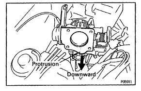
(b) Install a new gasket on the throttle body, facing thel protrusion downward.
