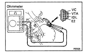
(e) Using an ohmmeter, measure the resistance between each terminal.
