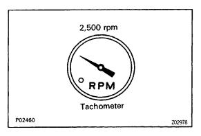
(b) Maintain the engine at 2,500 rpm.
