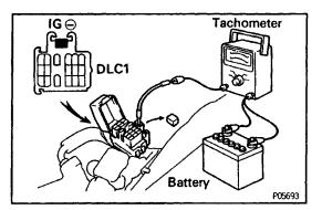
2. With a tachometer connected to the system, connect the test probe of the tachometer to terminal IG (–) of the data link connector 1.
