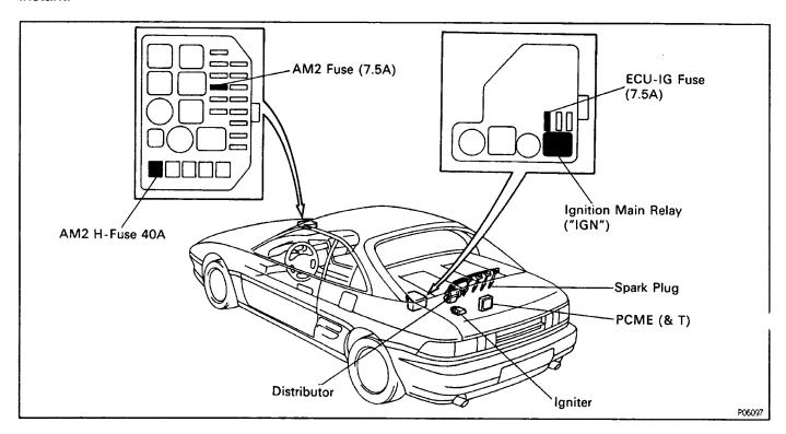
The PCME (& T) monitors the engine condition by signals from each sensor, calculates the ignition timing andsends an ignition signal to the igniter. High voltage from the ignition is distributed to each spark plug in the appropriate order to generate a spark between the electrodes, which ignites the air–fuel mixture.
