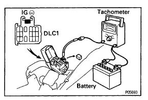
2. With a tachometer connected to the system, connect the test probe of the tachometer to terminal IG (-) of the data link connector 1.
