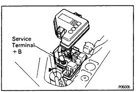
3. With a tachometer connected to the system, connect the power source probe of the tachometer to service terminal +B of the engine compartment relay box.
