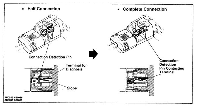
HINT: The illustration shows connector (6). Connectors (1) and (2) also have the same operating principle.
