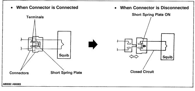
HINT: The illustration shows connectors (4) and (5). Connector (1) has a short spring plate on the female terminal side, but the operating principle is the same.
