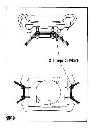
(1) Using 3 wire harnesses, wrap the wire harnesses at least 2 times each around the bolts installed on the left and right sides of the steering wheel pad.
