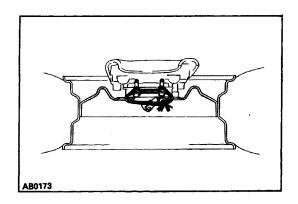
(2) Face the upper surface of the steering wheel pad upward. Separately tie the left and right sides of the steering wheel pad to the disc wheel through the hub nut holes.
