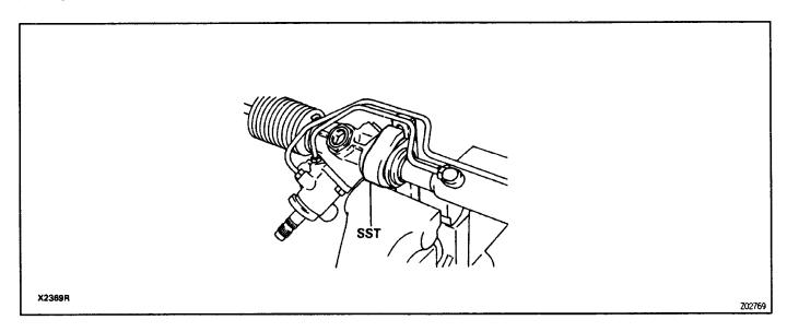
The oil seals on both sides of the power cylinder are for the prevention of leakage of the high pressure fluid which acts on the piston. Always use new oil seals when reassembling and be very careful not to scratch or damage them.
