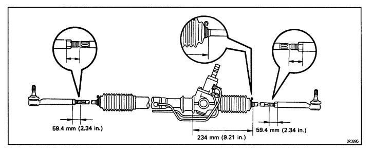
HINT: The dimension of the tie rod end is a reference value, so always adjust the toe-in before tightening the lock nut.
