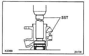
(c) Using SST, press in a new bearing. SST 09620–30010 (09631 –00020), 09630–24013 (09620–24020)
