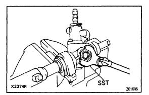
**6. REMOVE RACK GUIDE SPRING CAP LOCK NUT** Using SST, remove the rack guide spring cap lock nut.
