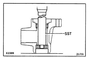
3. IF NECESSARY, REPLACE CONTROL VALVE LOWER BEARING AND CENTER BEARING (a) Using SST, press out the lower bearing. SST 09620–30010 (09631 –00020)
