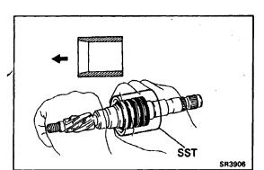
(d) Coat the teflon rings with power steering fluid, and carefully slide the tapered end of SST over the teflon rings to seat the rings.
