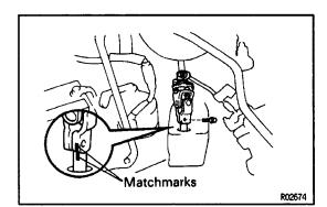
(b) Align rnatchrnarks on the universal joint and control valve shaft and connect them.
