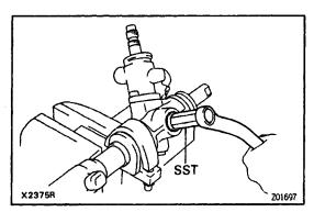
**7. REMOVE RACK GUIDE SPRING** Using SST, remove the rack guide spring cap. SST 09612–10131
