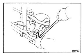
(d) Remove the two bolts and ball joint from the steering knuckle.
