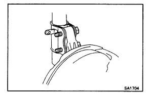
**7. REMOVE STEERING KNUCKLE WITH AXLE HUB** Remove the two bolts and washer–s, and remove the steering knuckle.
