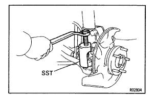
(c) Using SST, disconnect the tie rod end from the steering knuckle.
