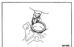
(b) Using snap ring pliers, install the hole snap ring.
