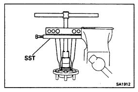
(b) Using SST, remove the hub bearing inner race (outside) from the axle hub.SST 09950–20017
