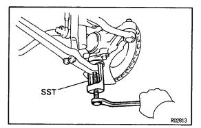
(b) Using SST, disconnect the lower arm from the ball joint.
