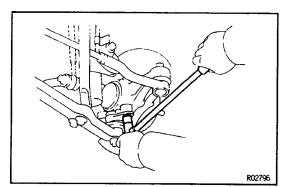
**3. REMOVE BALL JOINT FROM AXLE CARRIER** Remove the two bolts and ball joint.
