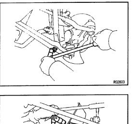
**3. DISCONNECT STRUT BAR FROM LOWER ARM** Remove the two nuts and disconnect the strut bar from the lower arm.
