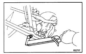
3. TORQUE STRUT BAR TO LOWER ARM Torque: 127 N-m (1,300 kgf-cm, 94 ft-lbf)
