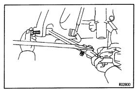
(b) Temporarily install the lower arm to the body with the washer and bolt.
