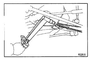
(c) Torque the bolts with the vehicle load applied on the suspension.
