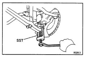
(b) Using SST, disconnect the lower arm from the ball joint.
