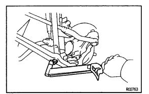
(b) Install the strut bar to the lower arm with the two nuts.
