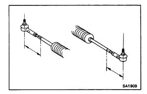
If wheel angles differ from the standard specifications, check to see of the lengths of the left and right tie rods are the same.
