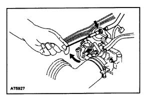
THROTTLE CABLE THROTTLE CABLE REMOVAL 1. DISCONNECT THROTTLE CABLE FROM ENGINE Disconnect the cable from the throttle linkage. 2. DRAIN TRANSAXLE FLUID
