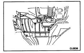
3. REMOVE NO.1 ENGINE UNDER COVER 4. REMOVE PARK/NEUTRAL SWITCH (See page AX-57)
