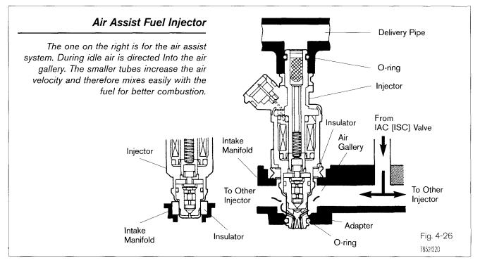
Inside the injector is a solenoid and needle valve. The fuel injector circuit is a ground switched circuit, To turn on the injector, the ECM turns on a transistor completing a path to ground. The magnetic field pulls the needle valve up overcoming spring pressure and fuel now flows out of the injector. When the ECM turns off the circuit, spring pressure will force the needle valve onto its seat, shutting off fuel flow.
