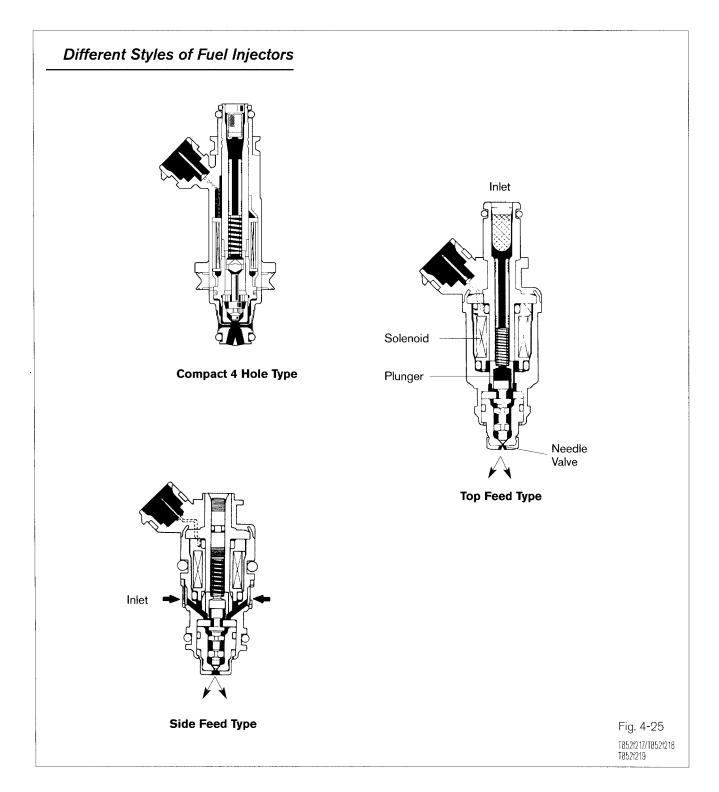
Different engines require different injectors. Injectors are designed to pass a specified amount of fuel when opened. In addition, the number of holes at the tip of the injector varies with engines and model years. When replacing an injector it is critical that the correct injector be used.
