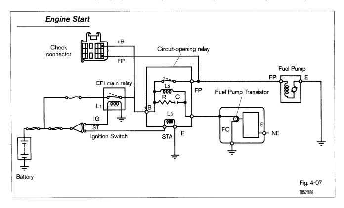
The following describes the basic methods of fuel pump control. An essential point to remember is that the fuel pump operates only when the engine is cranking or running.
